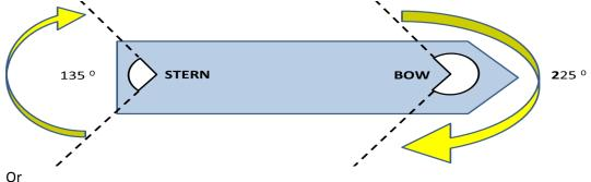
**B.** A white light attached to the vessel at or near the forward end displaying an unbroken arc of 225 degrees, and a white light attached to the vessel at or near the aft end displaying an unbroken arc of 135
